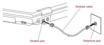
Figure 4-9 Connecting the internal modem
